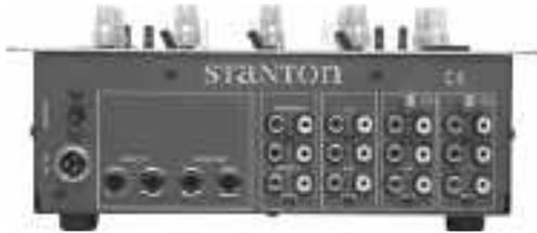
**Power:** This is the power switch to turn the mixer "ON" or "OFF"
